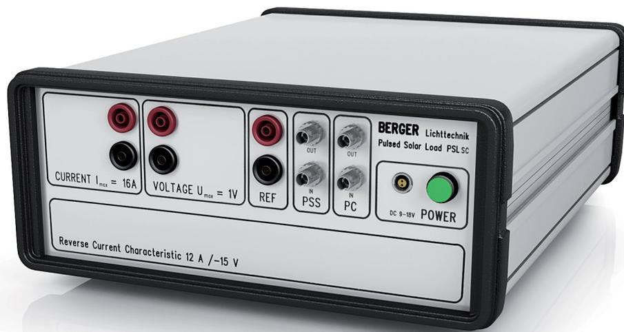
PC controlled load simulation and IV curve measurement for solar cells
